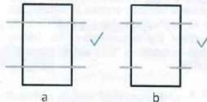
Fig. 3 Permissible alignment of mounting a : Parallel profiles for mounting; b: Parallel, aligned fingers of a mounting system.
