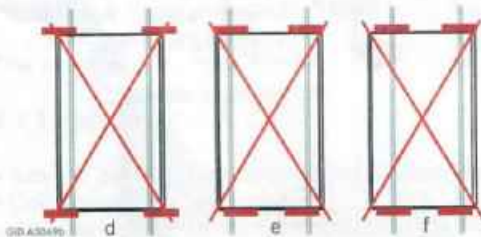
Fig. 7 Impermissible clamp arrangements (2) d: Protruding clamps, e: Opposing clamps have different distances to the PV module corners, f: Asymmetrical clamps on the short sides.
